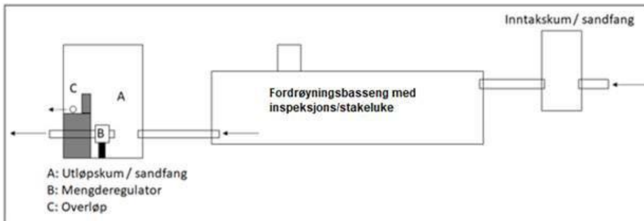
Figur 13. Prinsippskisse for fordrøyningsbasseng.
